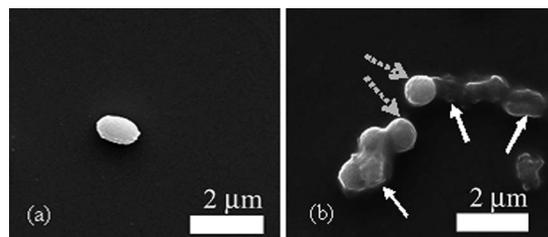
FIG. 5. SEM micrograph of PEMS sensor surface after exposure to (a) sample A  $-3.3 \times 10^3$  BA spores/ml, and (b) sample D  $-3.3 \times 10^3$  BA spores/ml with a  $3.3 \times 10^6$  cells/ml of SA and PA mixture. The solid arrows in (b) indicate BA spores which are cigar-shaped as shown in (a) while the dashed arrows indicate SA cells which are spherical.
